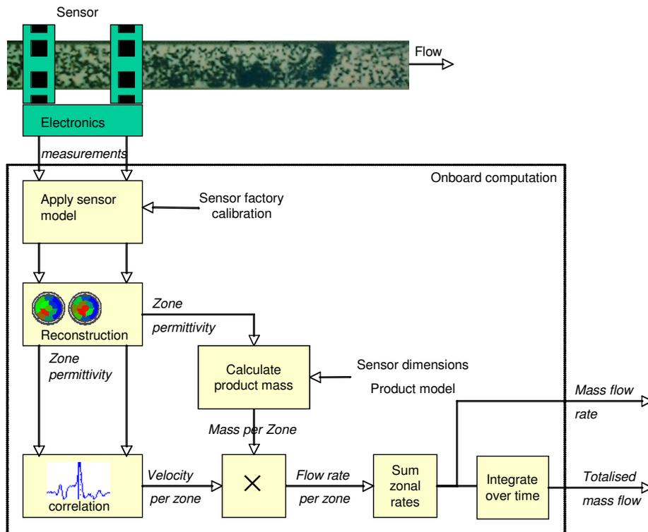
**Figure 1. Tomoflow Flow Analysis system**
