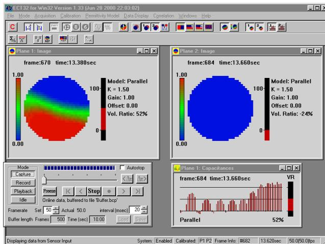
**ECT32-3.** ECT32-3 is a comprehensive on-line software suite for controlling and processing data from Tomoflow and PTL ECT systems. The software runs on the Windows operating systems. The images can be shown on the screen in real-time, then recorded and played back at user-defined speeds. Data files can be used for flow analysis using *Flowan\**.
