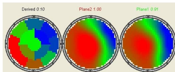
Flowan can calculate a number of average parameters for each zone, including average concentration and average flowrate. The example shows average concentration (left) over several 10s of seconds, compared with the instantaneous images (middle & right).
