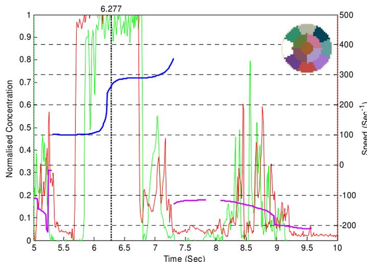
The velocity at each point in time within each zone is calculated by correlating the instantaneous concentration of one plane with the same zone in the other plane. The result is plotted as a second graph with axes in cm/second on the right hand side of the graph. The blue line shows positive velocities (in this case upwards) and the mauve line shows downward velocities. It can be seen in this case that the slug front is moving at 100cm/s but the tail is progressing at 300 cm/s.
