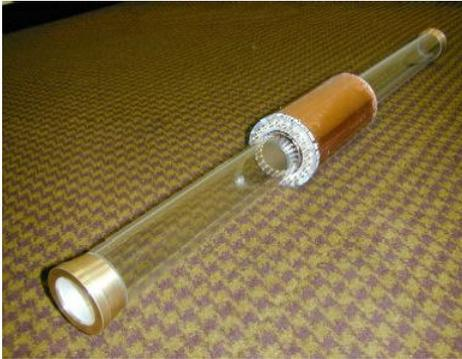
Data from the Tomoflow R5000 system may be saved to file for off-line flow structure analysis using Tomoflow's Flowan multiphase flow analysis software. Example results are given here for several flow conditions in a 50mm diameter pipe. The sensor used is a twin-plane unit with 3cm long electrodes axially separated by 10cm driven guard electrodes. The sensor is shown in the photograph mounted on a 50mm perspex pipe ready to be mounted in the test rig.
