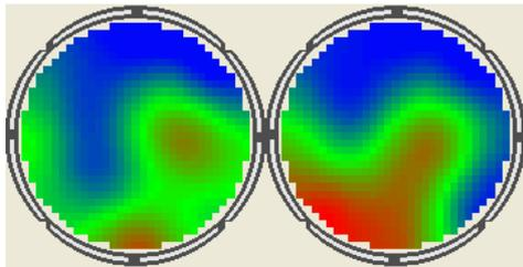
Images of flows are shown as circular maps with a grid of 32x32 pixels using a colour scale from blue (pixel empty) to red (pixel full). The example alongside shows the arrival of a slug front in a horizontal flow of plastic pellets in air. In this case the leading plane is on the right. Flowan automatically establishes the direction of flow .
