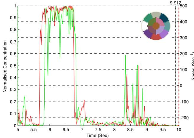
The first half of the graph shows upflow - an upward-going slug with concentration going from near 0 to near 1 in a short space of time at plane 1 (red line) slightly before arrival at plane 2 (green line). It can be seen that the rear of the slug is travelling faster than the front. On the second half of the graph the green line shows concentration events at plane 2 (upper) preceding their arrival at plane 1 (lower plane - red line).
