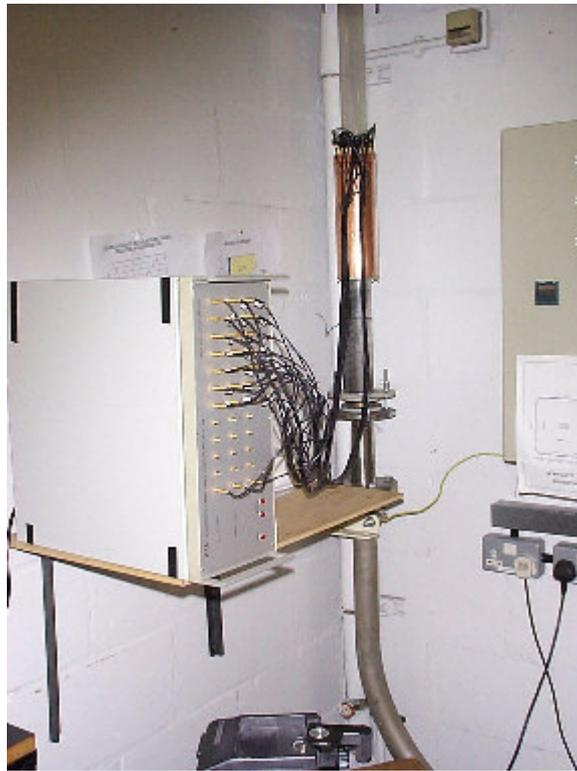
**Figure 3. ECT sensor in vertical section of flow rig**
