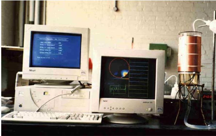
**An early ECT system imaging water droplets in kerosene.**
