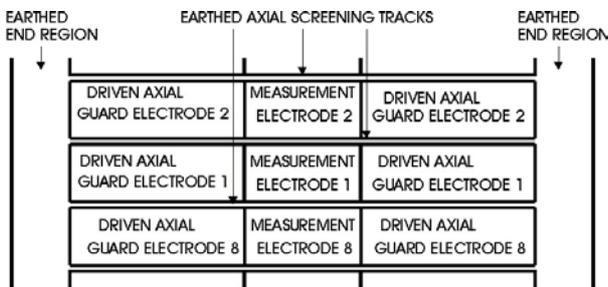
Figure 3. Partial PCB layout for an 8-electrode single-plane sensor
