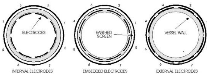
Figure 1 Circular sensor electrode configurations
