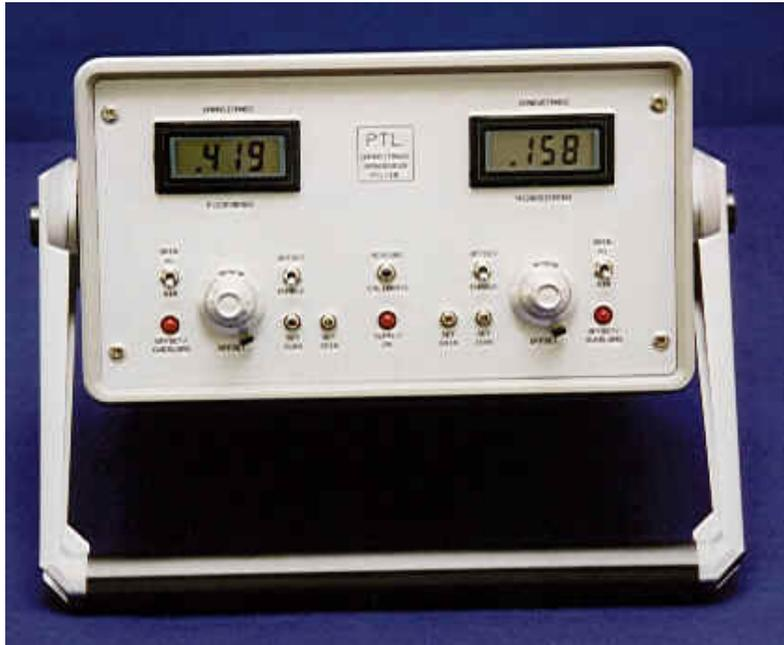
The PTL110 capacitance transducer measures small values of capacitance up to 10 picoFarads (pF) and parallel conductance up to 10 microSiemens (uS) in the presence of larger values of stray capacitance to earth. The measurement range can be extended to measure up to 100 pF and 100 uS with slightly reduced accuracy. Sets of both analogue and digital output signals are available..
